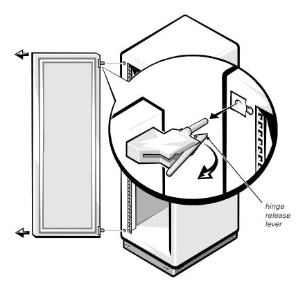
Figure 5. Removing the 42-U Rack Cabinet Doors
