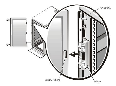
Figure 4. Removing the 24-U Rack Cabinet Doors
