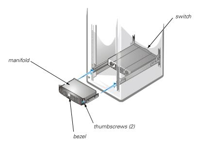
Figure 9. Installing the Manifold
