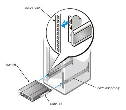
Figure 8. Installing the Switch Slide Assemblies
