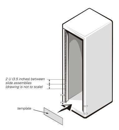
Figure 7. Using Template to Mark Vertical Rails
